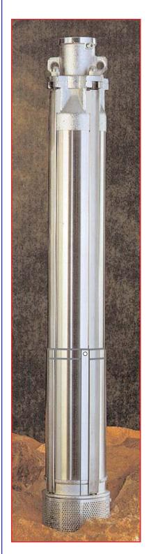
Multistage pumps designed specifically for 6" borehole and well applications, handling dirty water with entrained solids up to a max. 5mm diameter. They are suitable for pumped media temperatures up to 30°C with acidity ranging from 6 to 10 pH.
