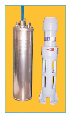
Progressive cavity (helical rotor) pumps designed for 4" borehole applications, handling clean or dirty water with entrained solids up to a max. 8mm diameter. Suitable for deep well applications from depths of 8m and more, they handle pumped media temperatures up to 30°C (larger motor/higher temperature models available) with acidity ranging from 6.5 to 12 pH.
