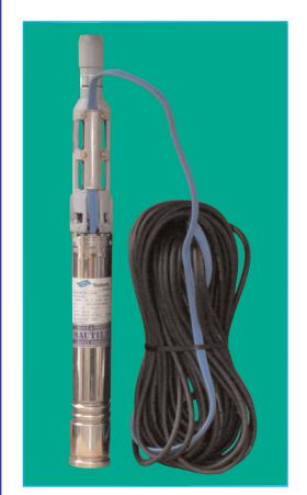
Progressive cavity (helical rotor) pumps designed for 3" borehole applications, handling clean or dirty water with entrained solids up to a max. 3mm diameter. Suitable for deep well applications from depths of 8m and more, they handle pumped media temperatures up to 30°C with acidity ranging from 6.5 to 8 pH. Supplied with 0.75kW, 400/3/50 motors with 35m H07RN-F cable as standard.
